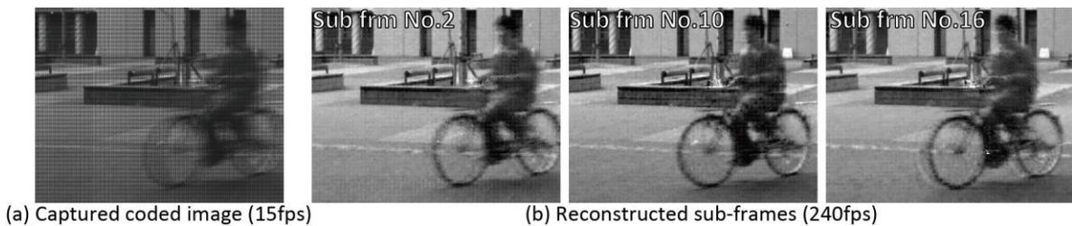
Fig. 4. **Real experiment.** the target scene is a cycling man. (a) shows the frame captured by the prototype QPE sensor (15fps). (b) shows three sub-frames from the reconstructed video (240fps).
