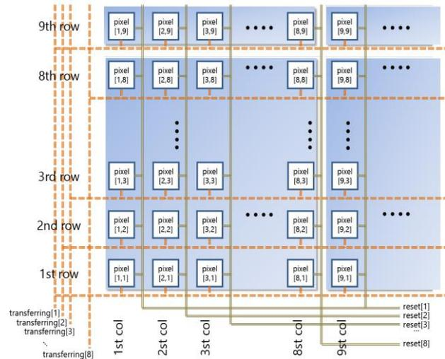
Fig. 2. Architecture diagram of CMOS image sensor with quasi pixel-wise exposure capability.
