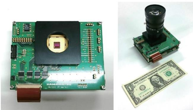
Fig. 1. Prototype CMOS sensor with quasi pixel-wise exposure.
