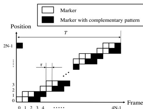
Fig.1 Time-space diagrams of an embedding method using a complementary set of markers. At least, one marker is always perfectly imaged with the method
