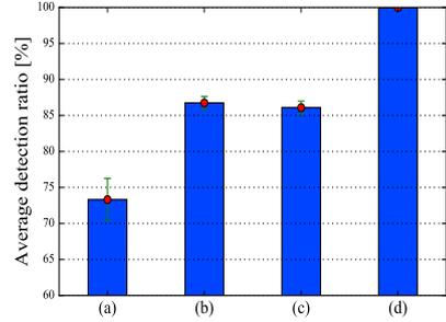
Fig.3 Average marker detection ratios. Error bars indicate  $\pm 3\sigma$  uncertainty. (d) is with the proposed marker arrangement, while (a)–(c) are not. (c) and (d) are with complementary patterns, while (a) and (b) are not.  $2N = 48$  for (a), while  $2N = 24$  for (b)–(d). (b) made the markers slightly perceptible by human while the others did not.
