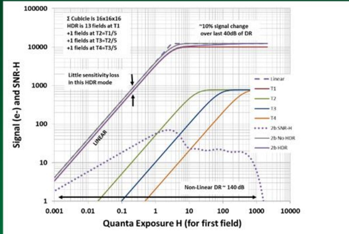
Alternate HDR mode that improves low-light sensitivity at expense of reduced SNRH at higher light levels. Note 10% of max signal change occurs over last 40 dB of DR. First 13 fields duty cycle is unity, next field duty cycle is 1/5, next field is 1/25, and last is 1/125. The contribution of each set of fields is also shown.
