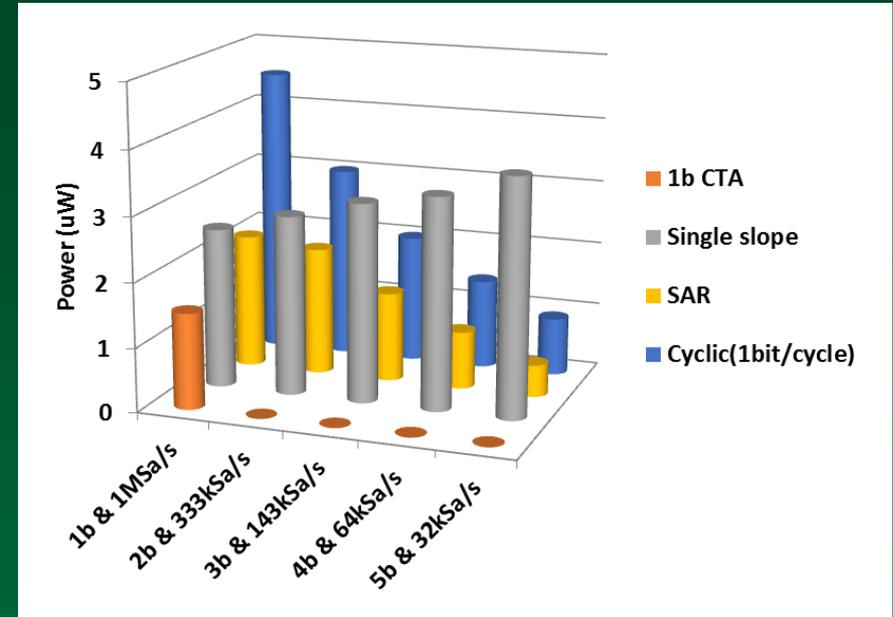
Power dissipation of single-bit and multibit QIS ADCs operating at different resolutions, and at different speeds for constant flux capacity. (From simulation of a chip in fab, S.Masoodian, D. Starkey, A. Rao, S. Chen, K. Odame and E.R. Fossum)
