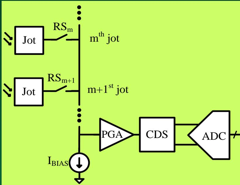
Block diagram of readout signal chain.
