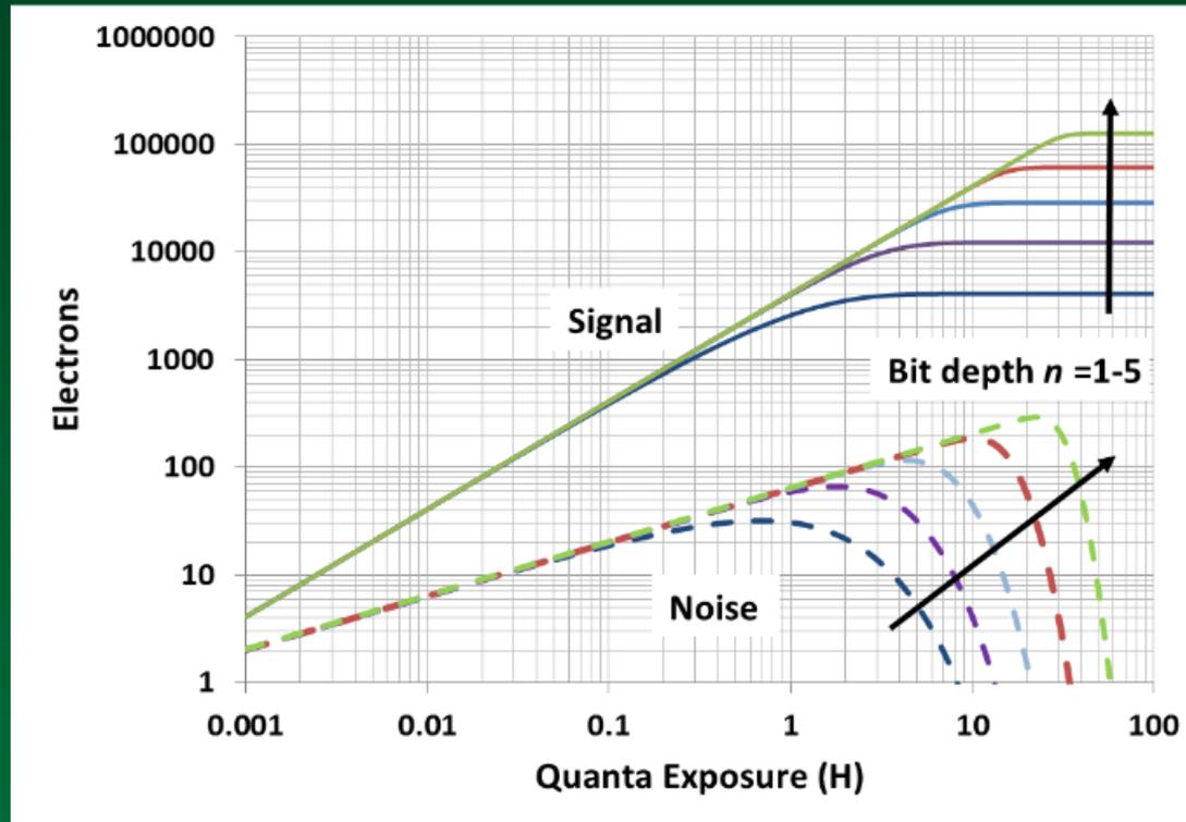
Log signal and noise as a function of log exposure for multi-bit QIS jots with varying bit depth. The signal is the sum over 4096 jots (e.g. 16x16x16). Saturation signal is  $4096 \cdot (2^n - 1)$ .
