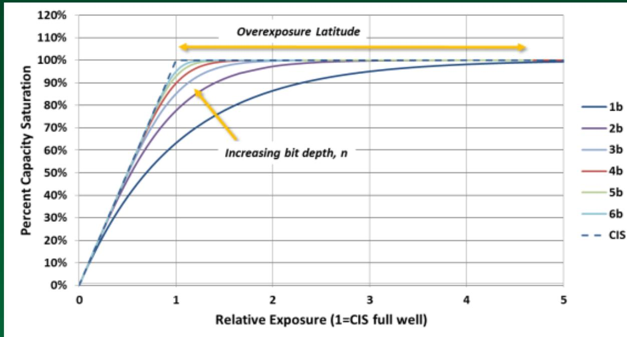
Non-linearity and saturation characteristics of single-bit and multi-bit QIS for  $1 \leq n \leq 6$  bits. For the QIS, the capacity of the full well is given by  $FW=2^n-1$ . The relative exposure is the quanta exposure  $H$  (in photoelectrons) divided by the full well, and the percent saturation is calculated from the expected number of photoelectrons in the photosite. Generally for the QIS, a “cubicle” in  $x,y$ , and  $t$  might be summed.
