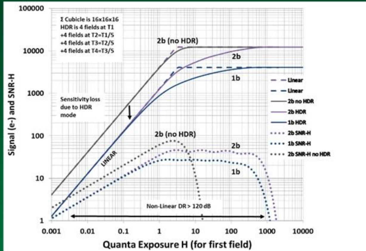
Comparison of an HDR mode for 1b and 2b QIS. Cubicle is 16x16x16 fields, with 4 different shutter duty cycles. First 4 fields duty cycle is unity, next is 1/5, next is 1/25, and last group of 4 fields is 1/125. Signal is sum of cubicle data
