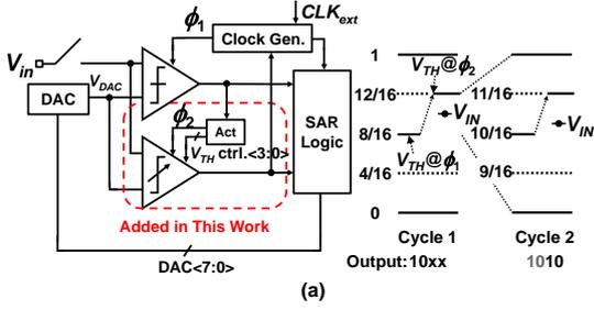
Fig. 4. 2bit/step SAR-ADC with dynamic threshold configuring comparator.
