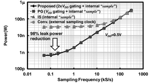
Fig. 7. Experimental results of leakage power reduction by self power gating.
