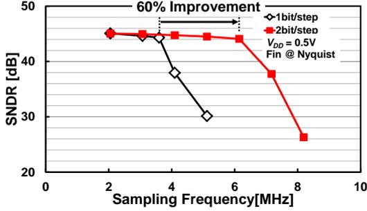
Fig. 5. Experimental results of speed improvement by 2bit/step.
