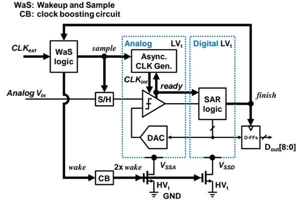
Fig. 6. Self-power gating technique to reduce leakage power.
