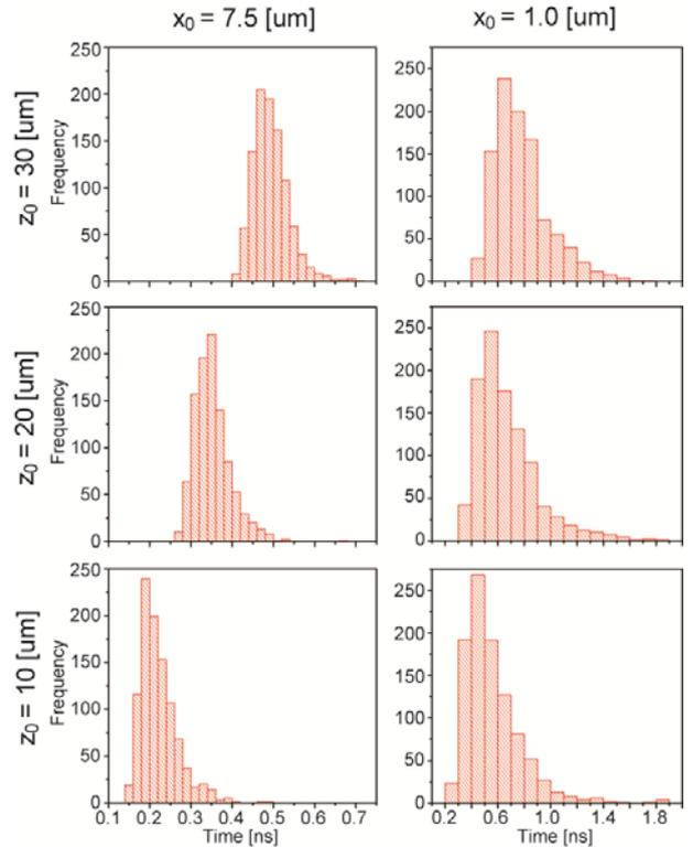
**Fig.2** Histogram of the traveling time of the photoelectrons.
