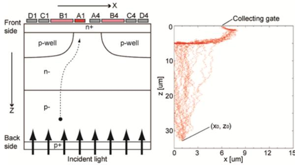
**Fig.1** Cross section of the multi-collection-gate image sensor (left), and an example of electron trajectories obtained from the Monte Carlo simulation (right).
