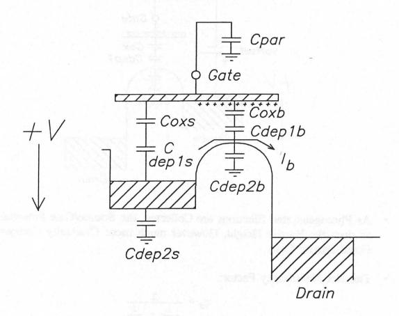
• As Collection Well fill up with Photogenerated Electrons, the Gate Potential is Pushed Up by the Series Combination of  $C_{oxs}$  and  $C_{depls}$ .  $C_{par}$  loads the Gate Electrode, therefore, it Should be Minimized
