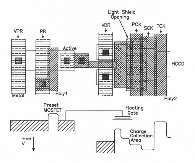
• The Floating Gate is Preset with the PR/VPR MOSFET Structure. Two Additional Gates PCK (Partition Clock) and TCK (Transfer Clock) are used to Enhance the Charge Collection Area.
