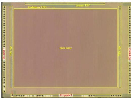
Fig. 11: Sony IMX214 13 MP Stacked CIS – CIS Die at Poly Level
