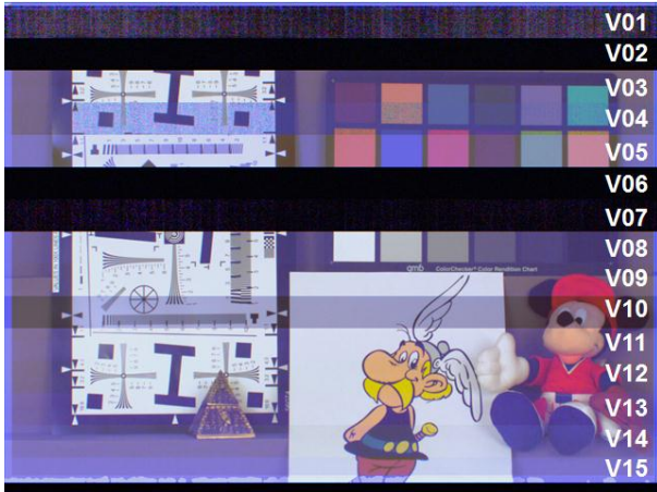
Figure 9: Picture taken with one P-type sensor for testing. The sensor integrates fifteen different pixel design variations each having more than 200000 pixels.
