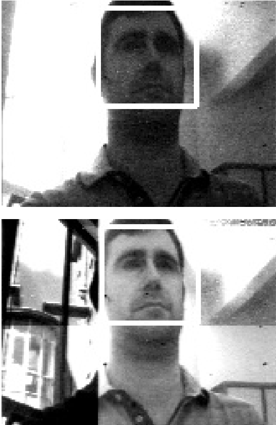
Fig. 2. Experimental results showing image capture with global adaptation (top) and ROI-driven adaptation (bottom).
