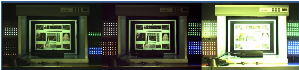
Figure 11. Lab set-up LEF and Flourescent flicker in ERS mode (left), no flicker LFM mode (middle), saturation ERS mode (right)
