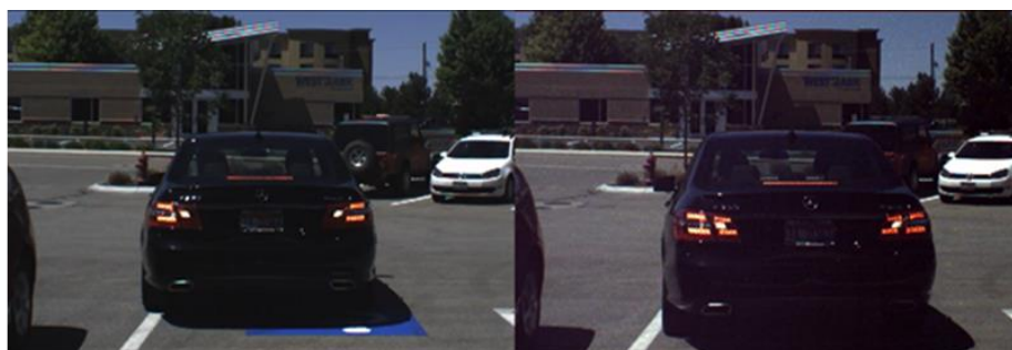
Figure 12. Outdoor car missed brake lights in ERS mode (left) captured in LFM mode (right)
