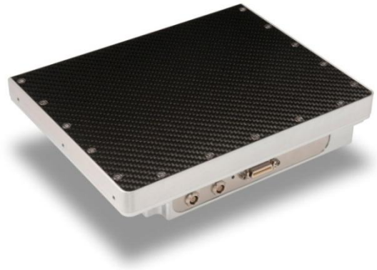
Figure 11 Photograph of a complete X-ray detector comprising a wafer-scale imager with the 14-bit ADC, scintillator layer for X-ray to visible light conversion and interfacing electronics
