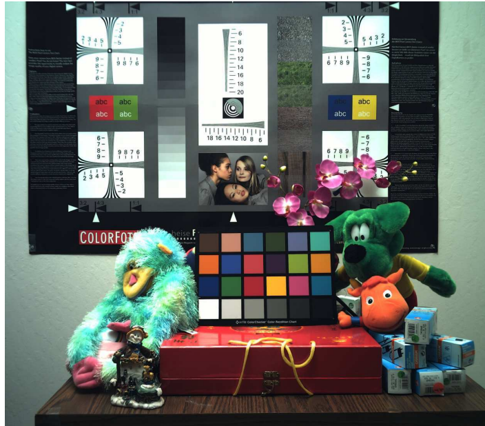
Figure 5. Color image from 1.1 \mu\text{m} , 5MP array, CIS stack chip (200 lux, 8x gain, 15 fps, f/2.4 lens)
