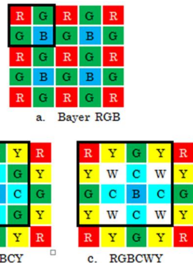
Fig.1. CFAs of the Bayer pattern and two proposed patterns with black square demarcating the kernel for each CFA
