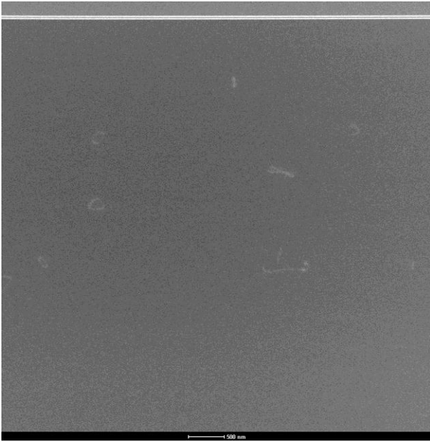
Figure 9. TEM microphotograph of RTA 1100°C 30sec (some dislocations are observed.)
