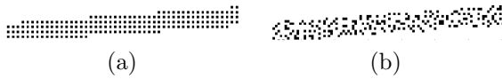
Figure 4: Examples of slant line representation with (a)conventional pixel placement and (b)pseudorandom pixel placement.
