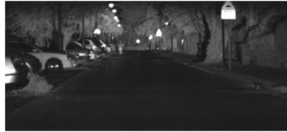
Figure 8. AGIS imagery at night. A pedestrian is clearly seen at a range of 115 meters.
