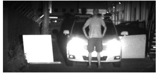
Figure 5. Vehicle with high headlights and a road sign are located 20m from the AGIS.
