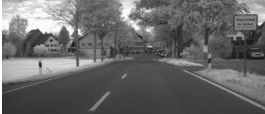
Figure 10. AGIS raw imagery at day-time. Images are taken with a narrow band filter at 800nm and there is no active illumination.
