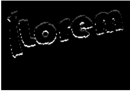
Figure 8 – Frame difference-based motion detection image from a moving text captured at 1000 FPS
