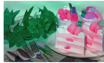
Fig. 4. In a 0 lx no-visible-light environment, a color image has been reproduced with only NIR illumination using the camera.
