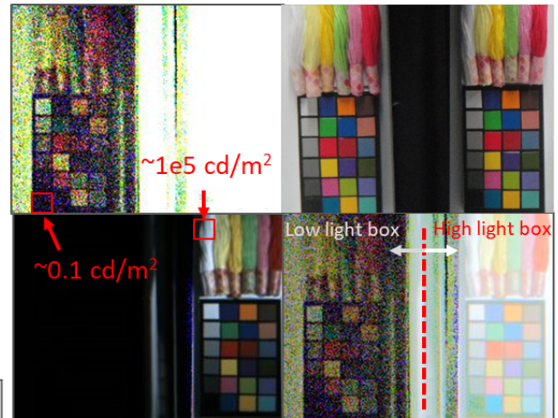
Fig.8 100dB HDR image in multiple exposure of 6 and 0.6msec. (top,right : An object, top,left : HCG / long exp, bottom,left : LCG / short exp, bottom,right : 8bit HDR image)
