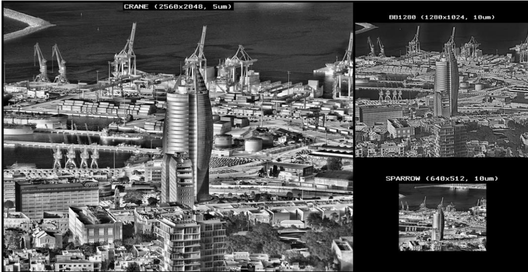
Fig. 6. Comparison of the view of Haifa Port in 3 formats: (1) SPARROW 640x512 at bottom right (2) BB1280 1280x1024 at top right and (3) This imager CRANE 2560x2048 on the left
