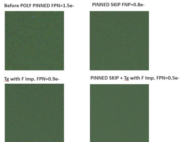
Fig.4. The PRNU comparison of twenty electron signal level at 32X sensor gain in low light illumination
