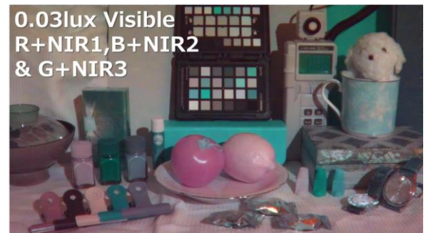
Fig. 5 Reproduced image with multi-NIR color image processing.
