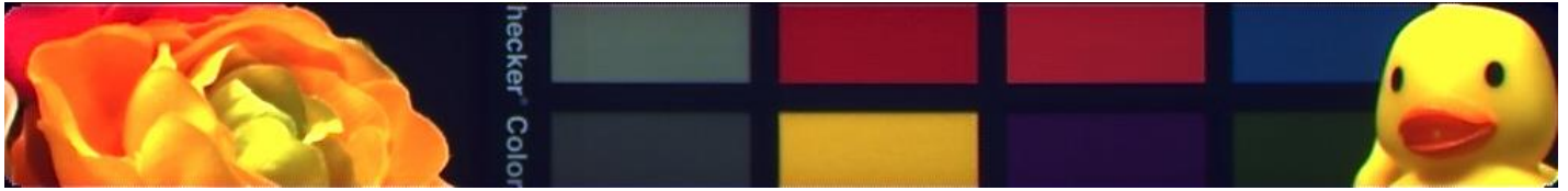
Figure 6: Sample Image captured with sensor. Left half of pixel array contains pump gate pixels and right half is made of PPDs. Full Array size is 256 (V) x 2048 (H).
