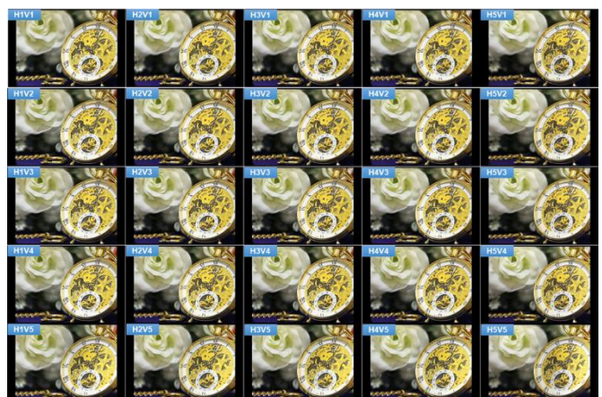
Fig.16 5x5 pentacosa-viewpoint images of the 5x1RGB+1x5G hetero penta-pixel image sensor.
