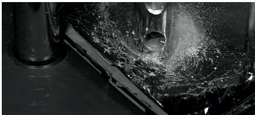
Figure 6 – Frame from a 100kfps video of cell-phone screen cracking
