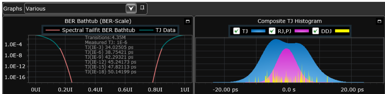
Figure 5: Serializer BER bathtub and total jitter histogram
