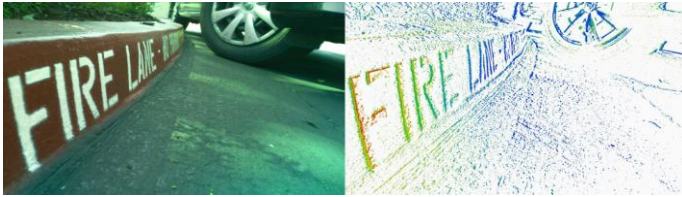
Fig. 11. Captured color image and corresponding signal phase/distance (close objects are reddish, distant objects are bluish).
