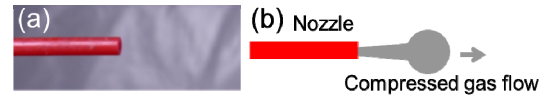
Fig. 3. Object, transparent gas flow sprayed from a nozzle. (a) Photograph, (b) schematic. #
