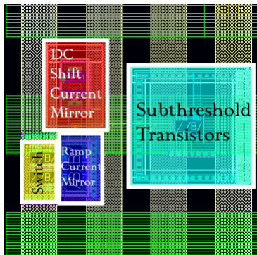
Fig. 9: Layout of logarithmic circuit. Dimensions: 8 \mu\text{m} \times 6 \mu\text{m}
