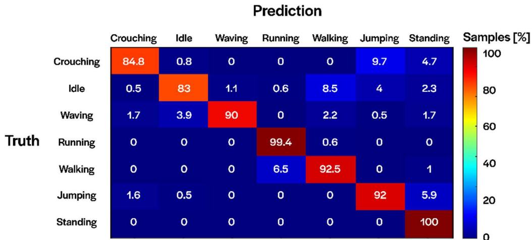
Figure 4: Confusion matrix of activities representing % of samples predicted in each class. Example: 1.6% of jumping data is confused with crouching down. Each class has approximately 200 samples.
