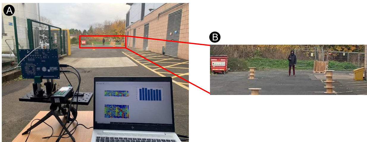
Figure 1. a) Picture of the camera setup. A 25 mm/f1.4 objective is used in front of the sensor, giving a 20 \times 5 degree field-of-view (FOV), together with a 10 nm ambient filter. Illumination is provided by a compact 850 nm VCSEL source with 10 ns pulse width and 60 W peak optical power triggered at 1.2 MHz. b) The FOV of the camera.
