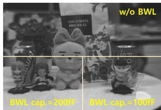
Figure 8. Captured sample image with BWL capacitor method.
