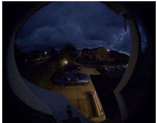
Figure 7: Outdoor images with local tone mapping of the 3MP sensor. Left: 2 ms integration time with direct sun light. Right: 30 ms integration time on a moonless night.
