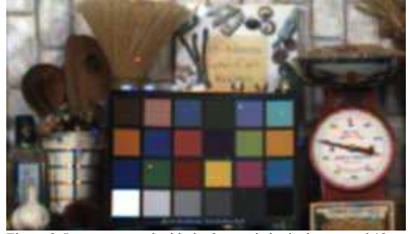
Figure 8. Image captured with the 3- \mu\text{m} -pitch pixel array and 12- \mu\text{m} -pitch photon counting circuit.
