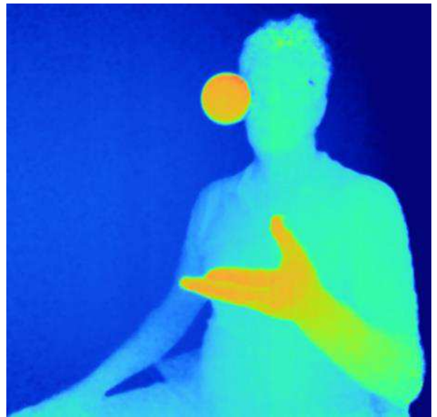
Figure 6- A depth image of a ball being thrown in the air, showing valid depth readout from the moving ball, highlighting the contribution of the in-pixel storage architecture to reduced motion artifacts.
