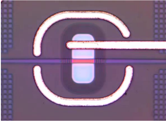
Fig. 3. Picture of the SPAD (from a newer production), showing the waveguides, the etched bottom cladding region and the metals for anode and cathode connections.
