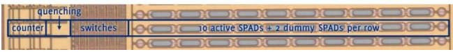
Fig. 3. Detailed view of the row architecture/layout with ten active SPADs plus two dummy SPADs per row. Here: layout variant BF.
