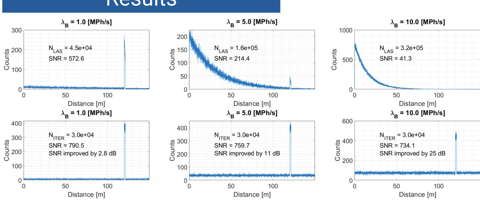
Simulation results: comparison of histograms from the standard detection approach (first hit - upper row) and linearized SPAD response (asynchronous time-gating - lower row). Thanks to the linearization over time, both range and SNR can be improved. The same number of laser shots has been considered for a fair comparison.
