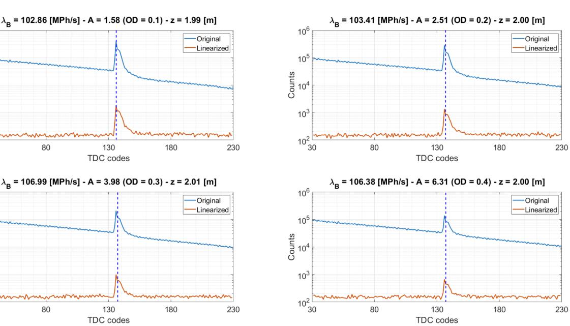
Ranging measurements at 2 meters distance with the ToF extracted thanks to the proposed histogram-less approach. The original and linearized histograms of timestamps are shown for reference. The background rate has been set beyond  $100\cdot10^6$  events/s and the measurements have been obtained with four different optical attenuation values for the returning laser intensity, to also demonstrate the effectiveness against pile-up distortion well beyond the standard 5% limit.
