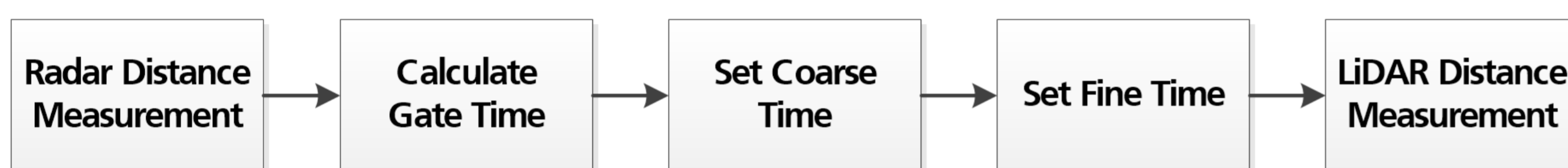
Fig. 1 Low-level fusion algorithm for the combination of LiDAR and RADAR. Coarse time corresponds is 6.25 ns (system clock) while fine time is stepped with 250 ps accuracy (delay line).
