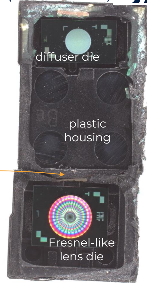
Plastic Housing w/ Diffuser and Fresnel Lens - Bottom View ©2024 Yole SystemPlus
