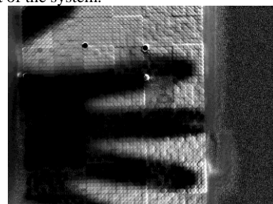
Figure 2 The amplified image by the avalanche image intensifier panel with a weak light ( \sim 1 \mu\text{W} ).
